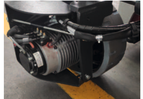
Motor electric AC; virare electrica pana la 90°
